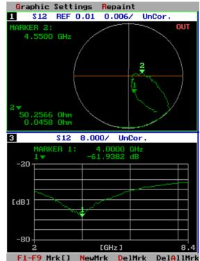
Graphic possibilities were also improved. Now it is possible to display a frequency difference  $\Delta f$  marker. Moreover sparameters of two different files can be displayed on the screen in the same time.
